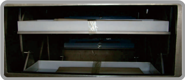
装于真空微波设备上的物料盘—采用聚苯乙烯材质，完全符合医用标准。 The material tray installed on the vacuum microwave equipment is made of polystyrene, which meets the medical standard completely
